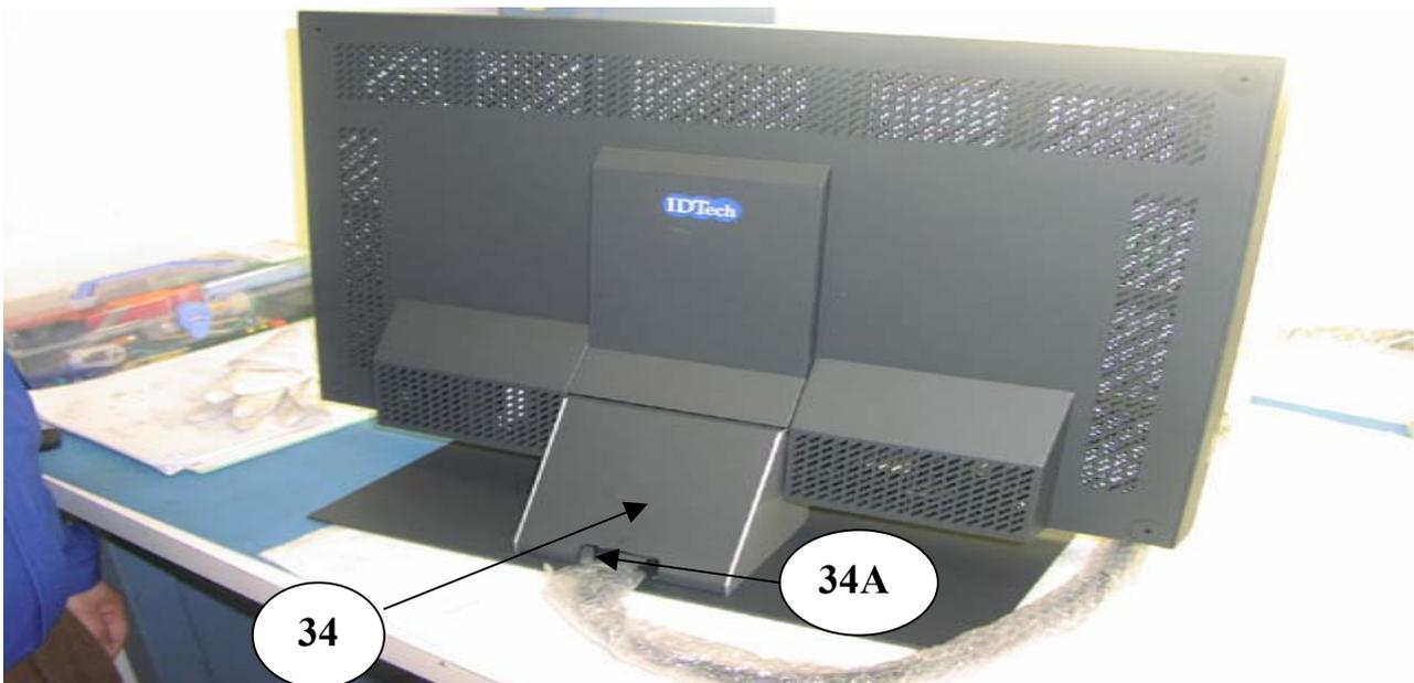
Install lower rear cover panel (Item 34) by snapping into position. Ensure interface cables routed through the opening (Item 34A). Monitor assembly is complete.
