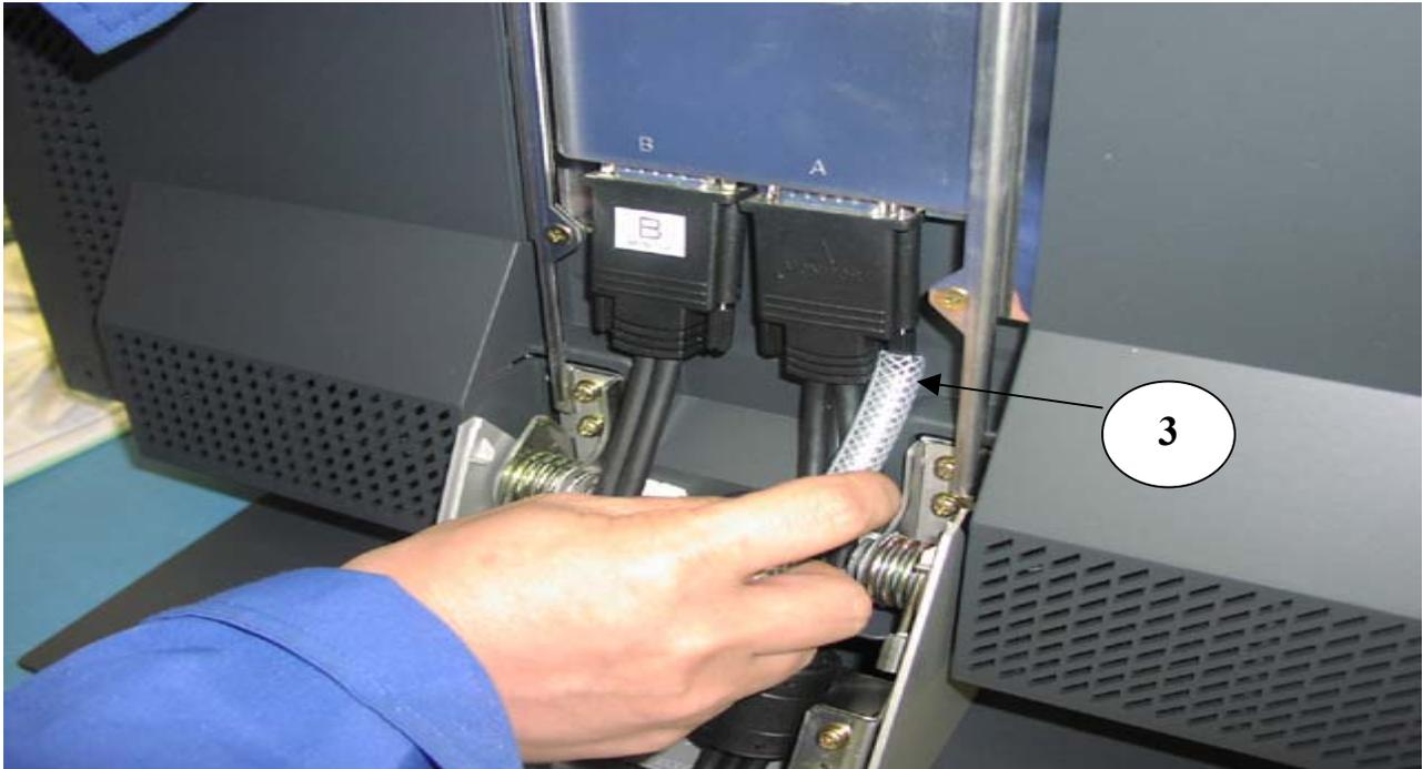
After second panel is removed, use a tube (Item 3) to loosen the four (4) connector mounting screws.
