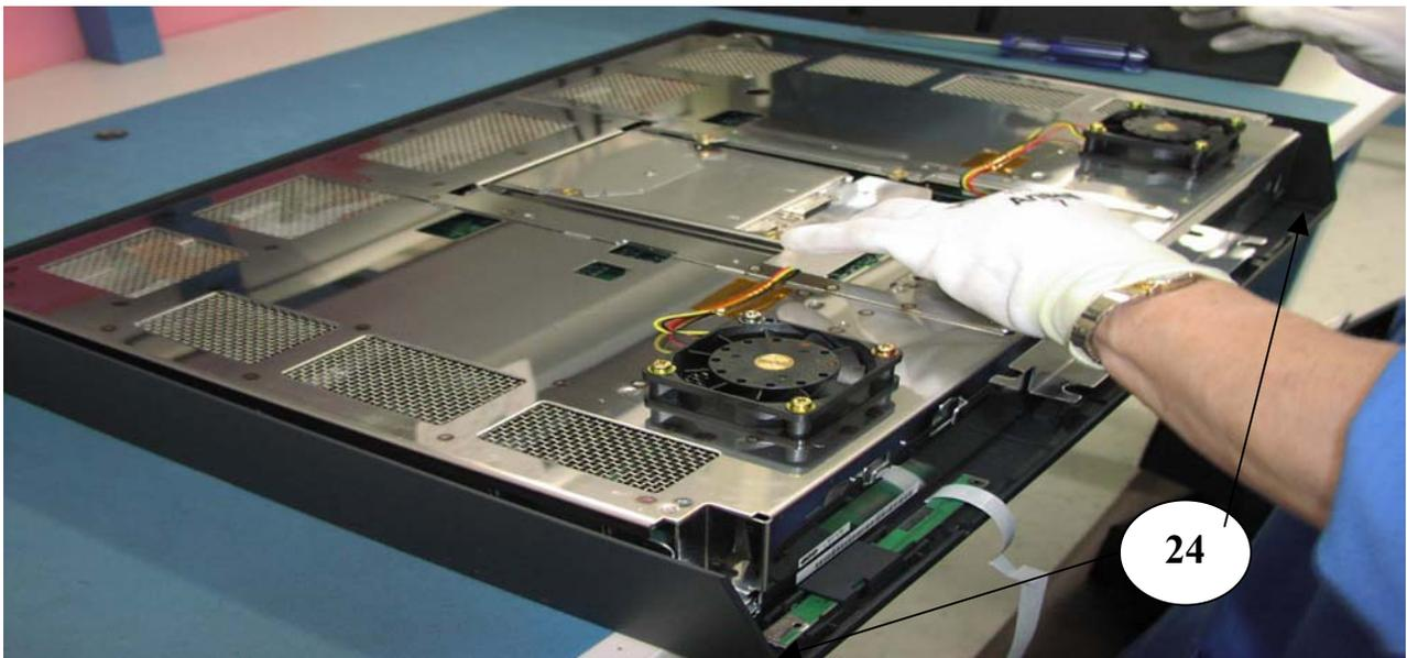
Lower backbone fully into the bezel, ensuring backbone is properly seated (Item 24).
