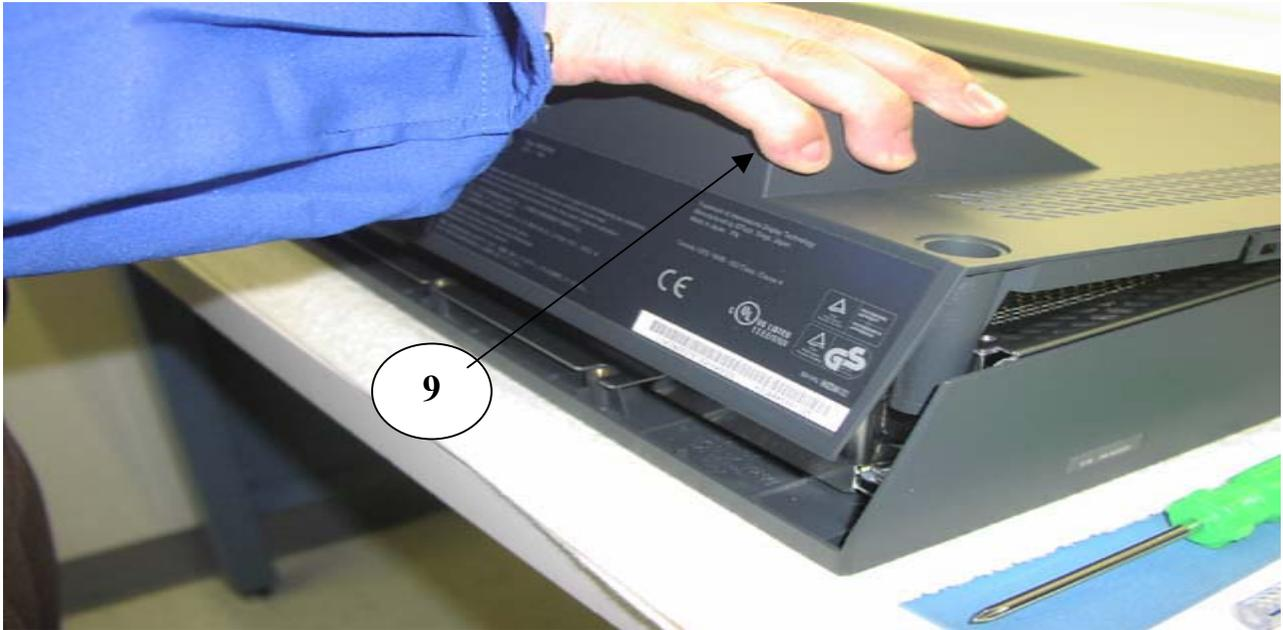
Grasp and unsnap rear housing (Item 9) by lifting until completely separated from monitor.
