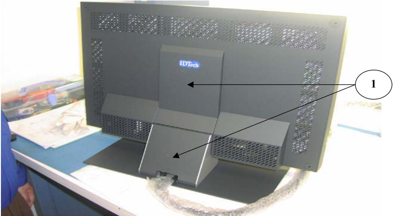
Situate monitor on workbench in preparation for removal of two (2) rear panels (Item 1)
