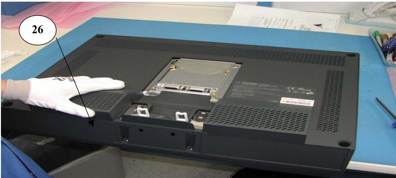
Place back cover (Item 26) onto panel assembly, ensuring cover is fully seated.
