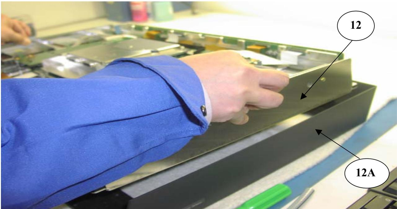
Lift and separate LCD module (Item 12) from monitor bezel (Item 12A).
